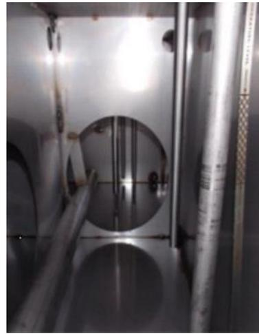
Even though the reservoir was previously cleaned at the factory, the customer requested IAS inspect and remove any remaining contamination. Only a very small amount of oil and soft contamination were found and removed by IAS.
