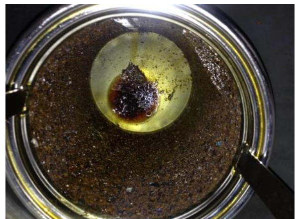
Solids removed from IAS multi stage bag filter was completely saturated with solids during C oil purification.
