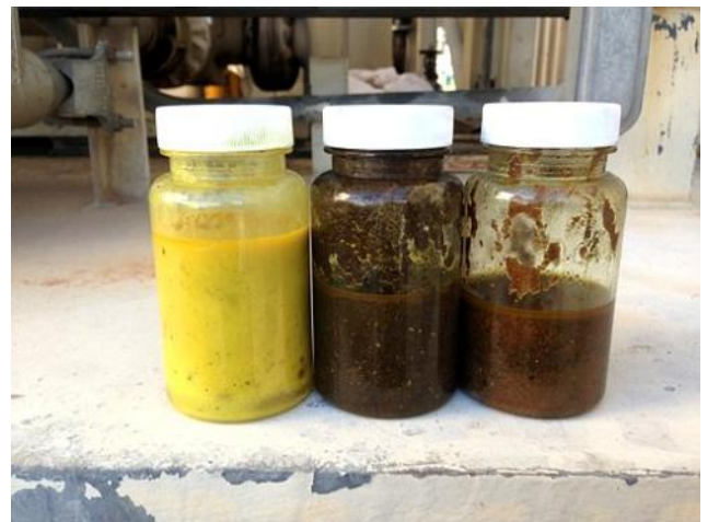
Bacteria, Water and Sludge Found in Reservoir
